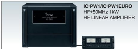
Covers all HF and 50MHz bands, provides clean, stable 1kW output. Automatic antenna tuner and compact detachable controller are standard. 2 exciter inputs are available.
